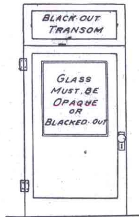
OUTSIDE DOORS WITH TRANSOM
